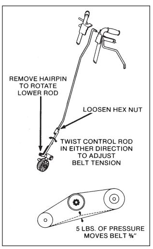
**Figure 4, Operator Presence Controls**
